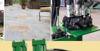
The **New Chris Cutter 3 twin cylinder** package delivers great value for the investment. This machine is ideal for cutting medium hard stones or thin stone into dimension. With the optional 24" high opening, stone can be placed on edge and cleaved or pealed with the bedding grain into flagging.
